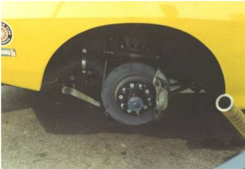
The Mercury rotor is bolted to the rear of the hub. Thus, a hat with sizeable offset is not needed. Photo: Mark Sorensen
