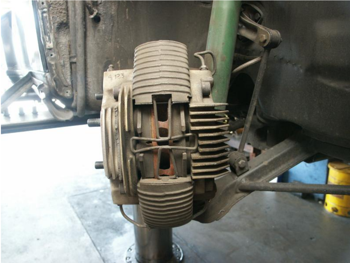
Yet another variation of the 917 Porsche caliper. The fins on the inboard puck housing are parallel to the ground. The fins on the outboard puck housing are perpendicular to the ground and the outward facing surface of the puck housing is machined smooth- probably for wheel clearance. Photo: A.J. Serrano
