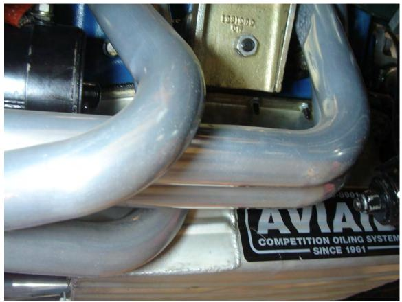
The headers fit precisely around the motor mount and next to the Aviaid oil pan. Photo: SRS
